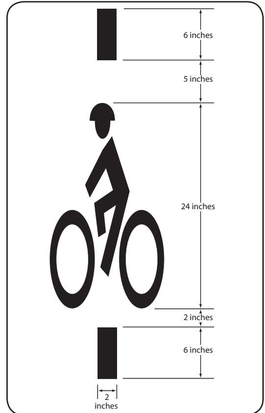
Recommended loop detector marking design.
