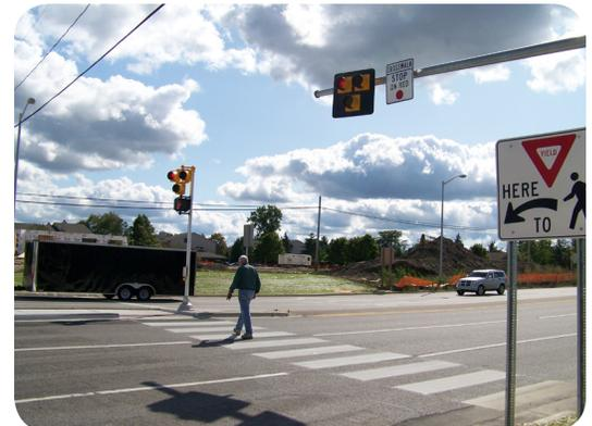
Pedestrian hybrid signal; also called HAWK signals (High-Intensity Activated Crosswalk).
