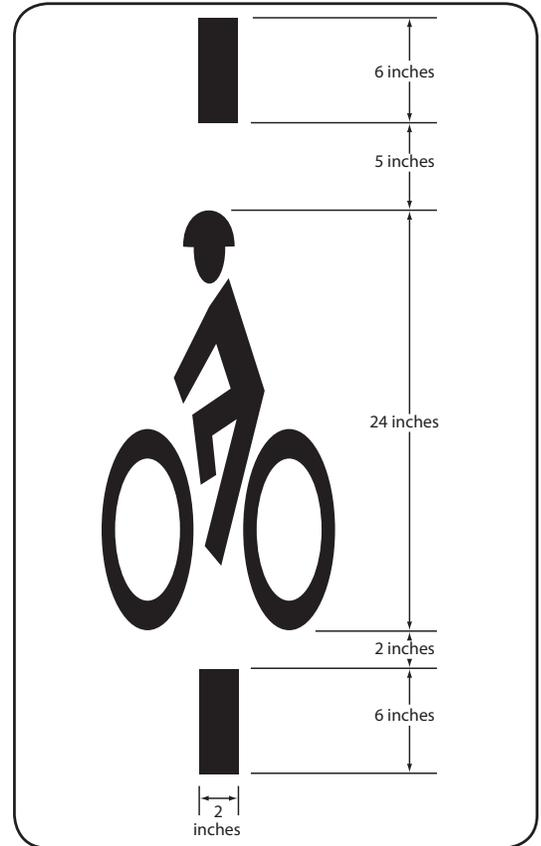
Recommended loop detector marking design.
